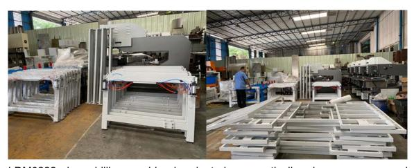
LDM0222 glass drilling machine is adopted pneumatically grip, sues upper and lower drill bits to drill holes, the lower drill can go up automatically, the position and speed can be adjusted. With automatic feeding function, the worktable can move up and down pneumatically. The machine can be used for continuous mass production and processing.
